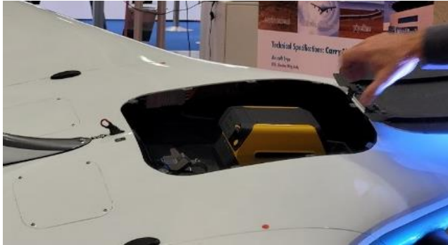
Fig 1. Installed Yellowscan Explorer
